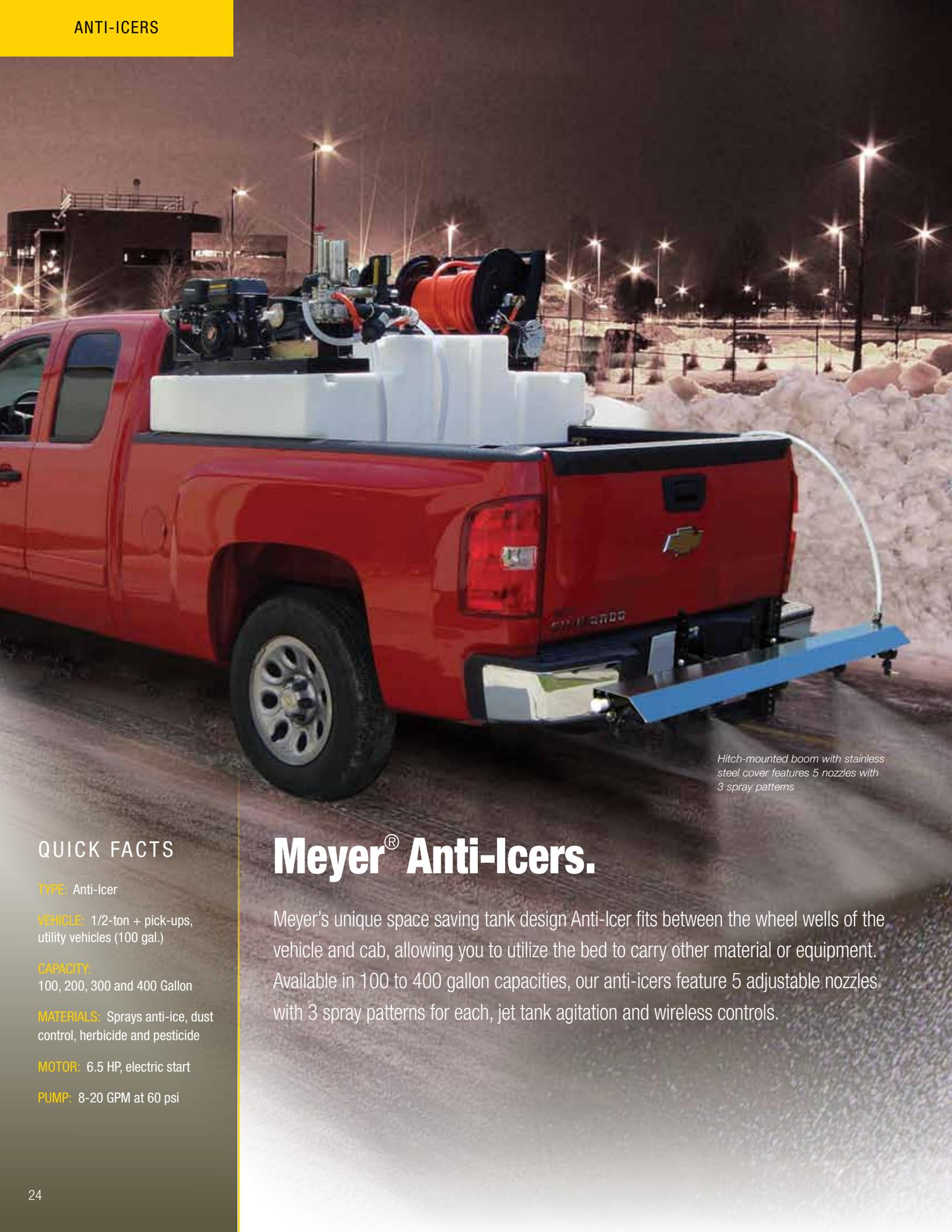
*Hitch-mounted boom with stainless steel cover features 5 nozzles with 3 spray patterns*
