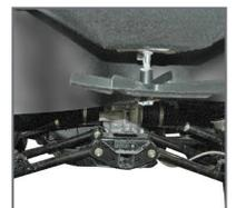
Impeller spinner shaft adjusts the spread pattern from 3'-4' to 8'-10'.
