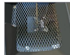
Internal filtering screen\* breaks up large clumps of material.
