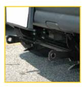
When dismounted, the Meyer Drive Pro mounting bracket leaves the front of your vehicle with a clean, neat appearance. The easy-to-use jack and pull handle system allows you to attach or detach the moldboard in seconds.
