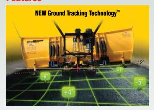
Allows the plow to automatically pivot up to 12° and stay engaged with uneven surfaces, so you can clean in just one pass. Ground Tracking Technology also allows the plow to remain level during transport and keeps the mount straight when mounting/dismounting on uneven surfaces.
