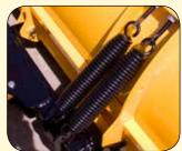
Heavy-duty trip springs last 2 to 3 times longer than the competition and are part of Meyer's ROC manufacturing process.
