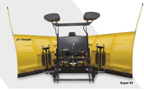
The Super-V3 and Super-V3 LD feature a bottom-trip design so only the lower portion of the blade gives way minimizing load loss. The bottom-trip feature also absorbs the shock caused by obstructions, saving wear and tear on the driver, truck and plow. Super-V3s also feature an exclusive upper-sealed center rubber deflector, along with optional wing deflectors to keep snow and ice off your windshield, and a lower-sealed center steel cutting edge to eliminate snow trails.
