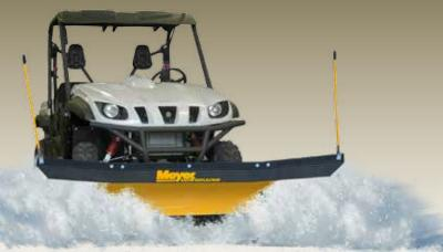
The dual flared wing moldboard design, coupled with the 65° attack angle, provides scoop and funnel discharge action.
