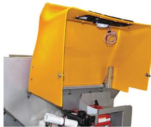
**Gas Springs\*\*** – The gas springs hold the engine shroud in the open position during refueling and maintenance.
