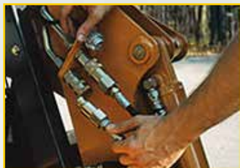
5 Attach the hydraulic couplers.
