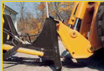
2 Position the attachment frame underneath the attachment flange.
