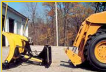
1 Align the attachment frame with the plow.
