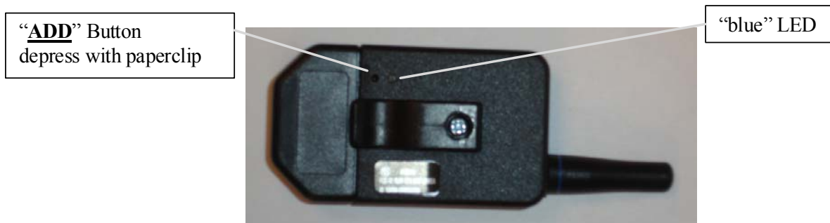
Fig. 2: Transmitter Back Button Assignments
