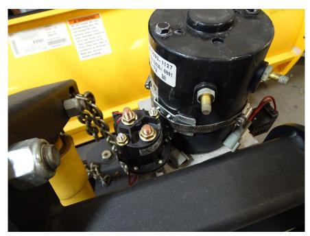
Step 3: Attach SOS Motor Cable (5) from the Motor Solenoid (2) to the hydraulic unit motor as shown.
