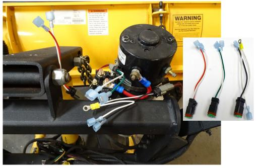
Step 5: Connect the three coil adapters (7) (red, green and black) to the Harness (4) (brown to white, red to red, black to black and green to green). Connect the heavy black wire to the motor ground as shown (A). If motor does not have a ground lug connect heavy black wire to the Hydraulic Block.
