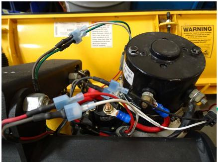
Step 6: Connect White wire loop to the small terminal nearest the hydraulic motor (A), the brown wire loop to the small terminal farthest from the hydraulic motor (B). Connect the heavy red wire to the large terminal of the motor solenoid (C).
